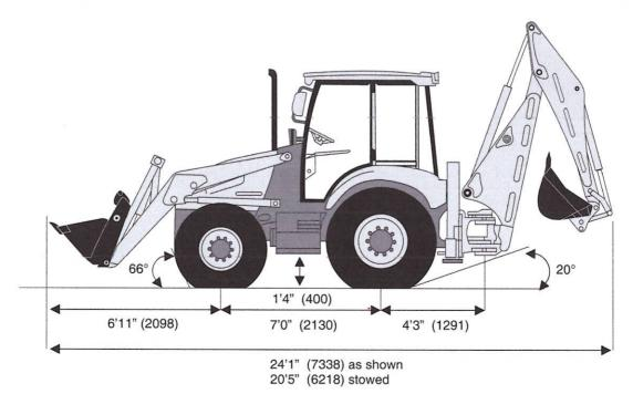
Note: Some dimensions will differ according to different tyre sizes, tyre pressures and loader bucket specifications
